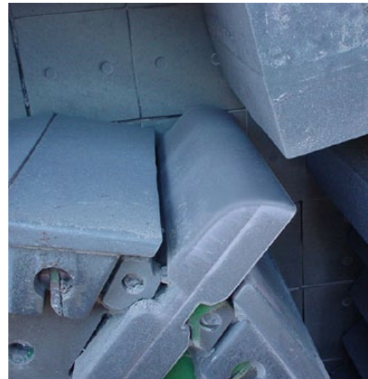
Re-sharpening of the striking bars in reverse operation.
