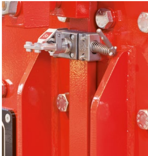
Key switch for crusher doors.
